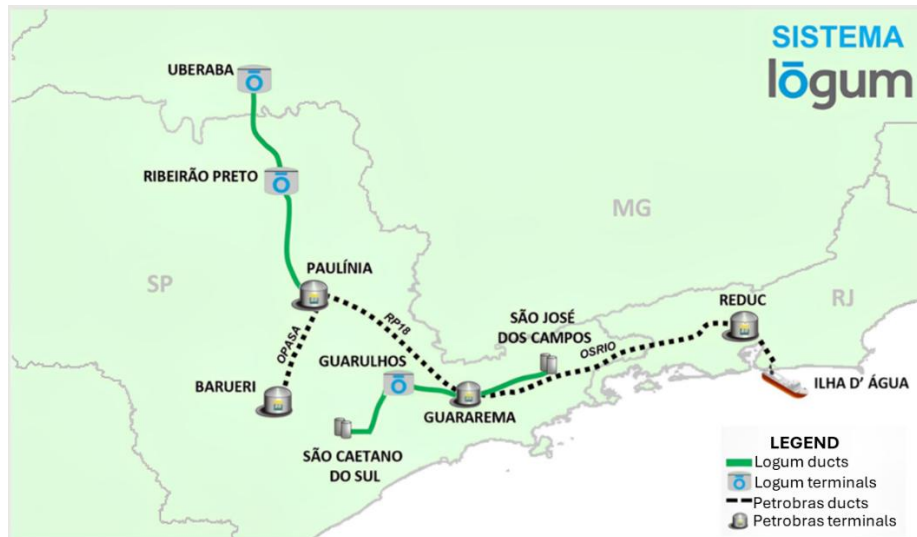
Figure 3 – Integrated logistics system for ethanol
